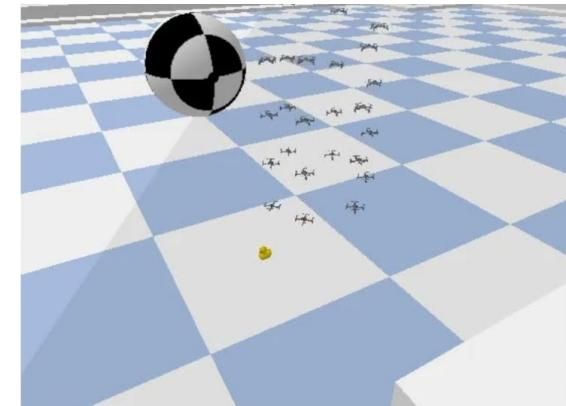
\* [gym-pybullet-drones](https://github.com/utiasDSL/gym-pybullet-drones) | PyBullet-based Gym for single and multi-agent reinforcement learning with nano-quadcopters ([utiasDSL.github.io](https://utiasDSL.github.io))
