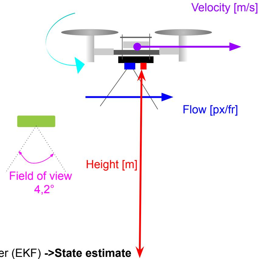
Measurement model -> Extended Kalman Filter (EKF) ->**State estimate**
